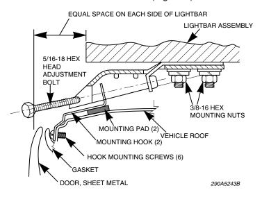
Figure 1: Lightbar attached to vehicle with hook kit
